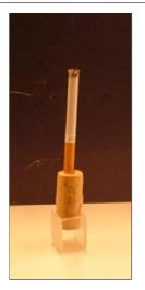
**Figure 6.** A glowing cigarette is attached to a piece of cork using a toothpick. If this is unstable, the cork may be squeezed into a holder.
