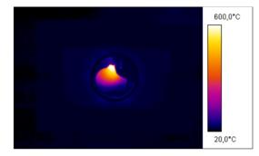
**Figure 12.** Infrared image directly after the explosion with surface temperatures at the top being above  $620 \degree C$ .
