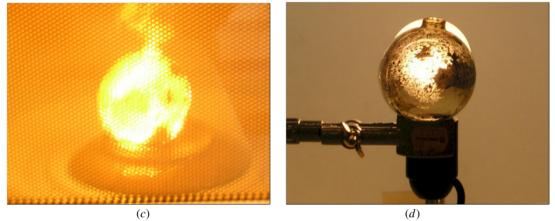
**Figure 3.** (*a*) Coated open glass sphere, usually used as a decoration on Christmas trees. Parts (*b*) to (*d*) correspond to the situation before (*b*), during (*c*) and after (*d*) treatment in the microwave. In the set-up of (*b*) and (*d*) the sphere is placed in front of an operating light bulb in order to demonstrate that in (*d*) a large part of the coating has evaporated, since the sphere has become transparent.
