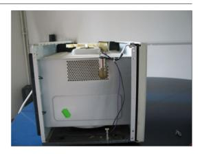
**Figure 7.** A microwave oven is illuminated by a light bulb behind a metal grid, e.g. at the side of the cavity (in this case, the microwaves are coupled in from the top).
