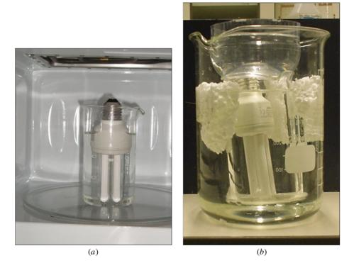
Figure 14. Set-up for studying the attenuation of microwaves by water with one or two beakers.
