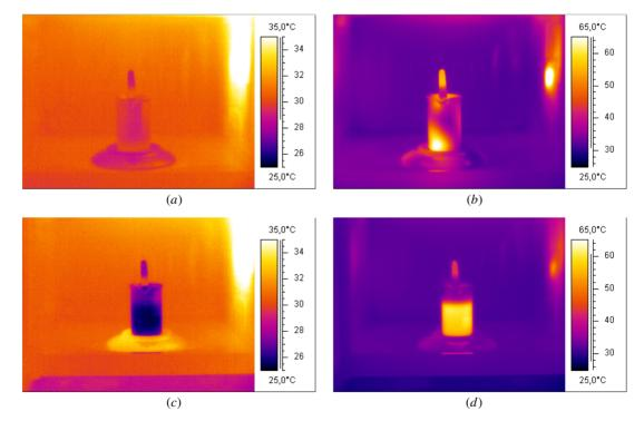
**Figure 5.** IR images of a spoon in a glass without water (top row) before (a) and after (b) heating, as well as with water (bottom row) before (c) and after (d) heating. Note the change in temperature scale between left and right.
