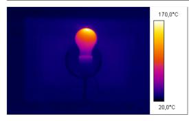
Figure 11. A 100 W light bulb after two minutes of operation.
