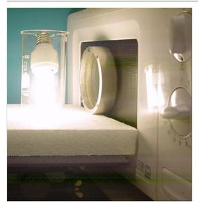
Figure 15. Discharge lamp in front of the modified microwave. The leaking radiation was strong enough to produce a discharge.
